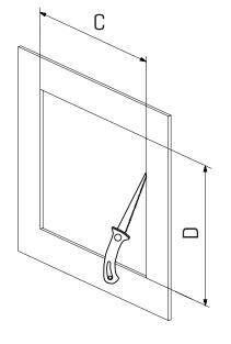
2 Trace around frame perimeter and through corner flange slots.
