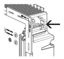
5 Place board into hole, clamping brackets to plasterboard by fastening 4x corner screws
