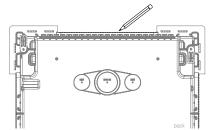
4 Rotate clips within confines of board
